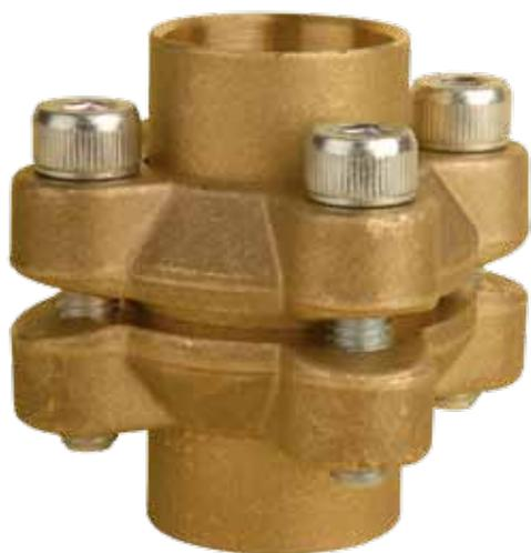
The sealing system between the end of a male connection and a Flare-ODS adapter allows avoiding the flaring process on copper tube end (national laws of some European countries don't accept this operation) because the tube end is brazed into the solder connection of the adapter. We wish to remember to our customers that they may assure no leakage of the male connection/adapter system only interposing the copper gasket 7580, supplied with the same adapter.
