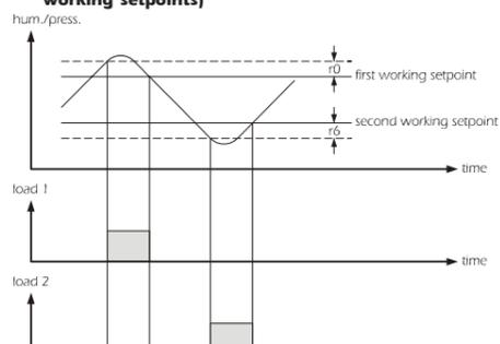
If parameter CFG has value 2, you can get each load to work with direct action (parameters r5 and r10 = 0) or with reverse action (parameters r5 and r10 = 1). In this example load 1 works with direct action and load 2 works with reverse action.
