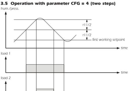
If parameter CFG has value 4, the second working setpoint will not be available and parameters SP2, r0, r6, r7, r8, r9 and r10 will not be significant.
