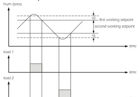
If parameter CFG has value 1, you can set the second working setpoint through parameter SP2 only (because it is relative to the first one). You can get each load to work with direct action (parameters r5 and r10 = 0) or with reverse action (parameters r5 and r10 = 1). In this example load 1 works with direct action, load 2 works with reverse action and the second working setpoint has a negative value.
