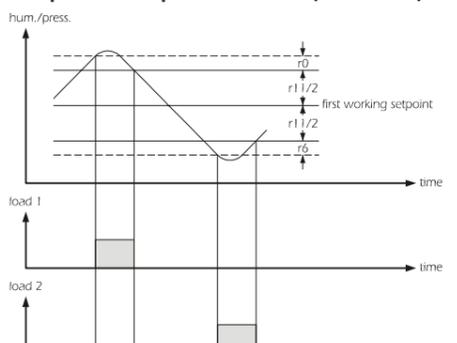
If parameter CFG has value 3, the second working setpoint will not be available and parameters SP2, r5, r7, r8, r9 and r10 will not be significant. Load 1 always works with direct action and load 2 always works with reverse action.
