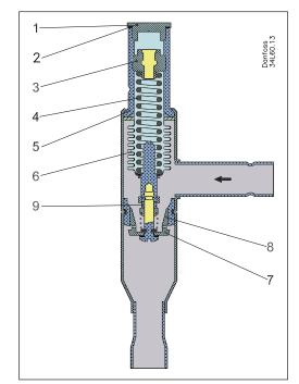
The hot gas bypass regulator KVC opens at a fall in pressure on the outlet side, i.e. when the pressure in the evaporator is beyond the set value.
