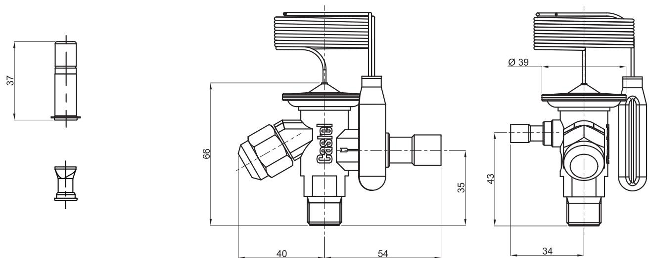
**TABLE 1A: General Characteristics of Body Assemblies of Liquid Charge Thermostatic Expansion Valves**
