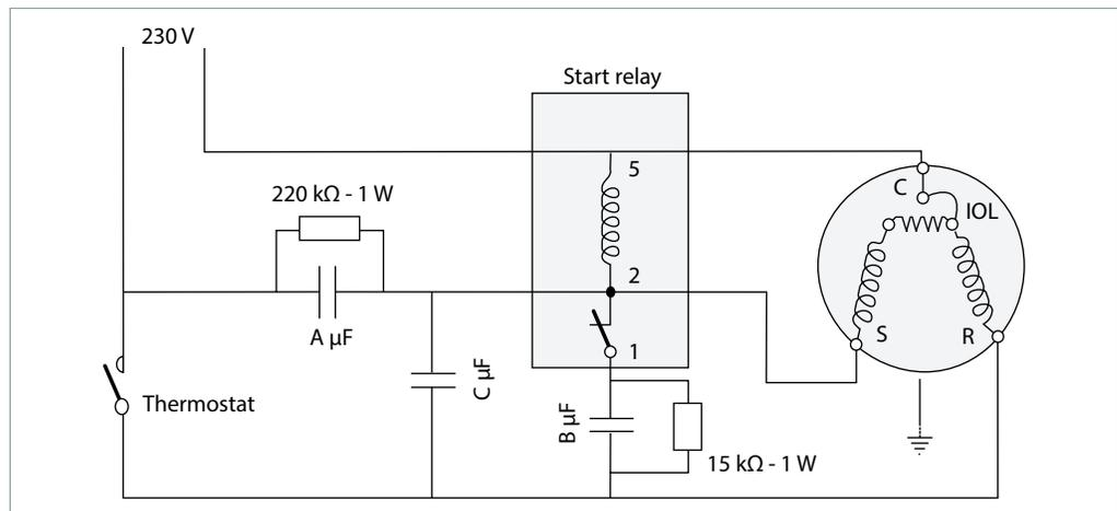
Single phase - CSR wiring without trickle circuit
