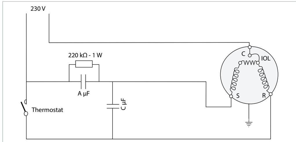
Single phase - CSR wiring with trickle circuit
