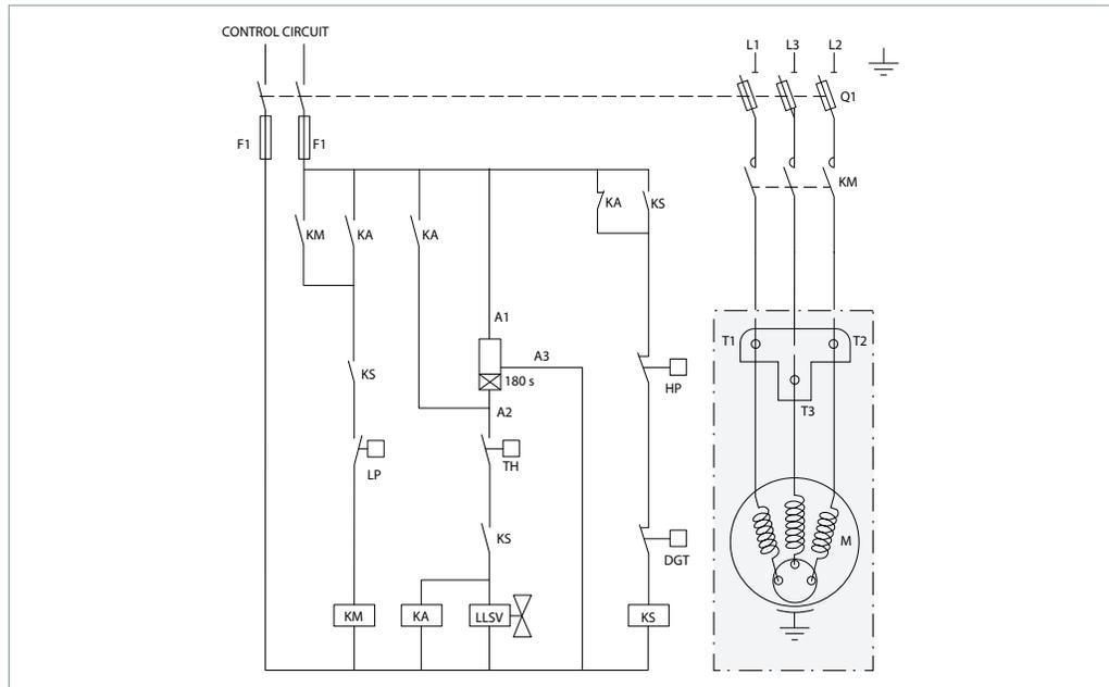
**Wiring diagram without pump-down cycle**
