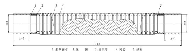
1. Copper bughStainsteel bausWhave hose4.Net hose5.Clamping ring
