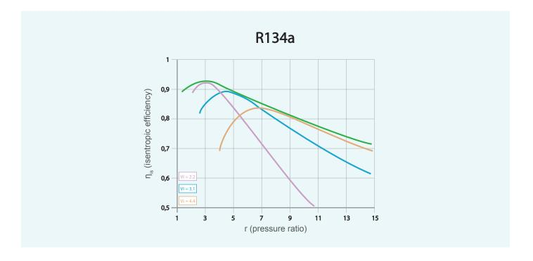
Since the geometry of the discharge port is generally fixed, the market offers different series of compressors to suit applications with different nominal pressure ratios. For instance Frascold offers two different main ranges of traditional screw compressors: the CXH and the CXW models, whose built-in volumetric ratios are 3.1 and 2.3 respectively and with which it is possible to cover a wide range of applications.
