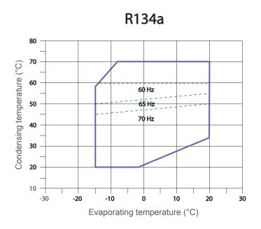
Suction gas superheating 10K - without liquid subcooling.
