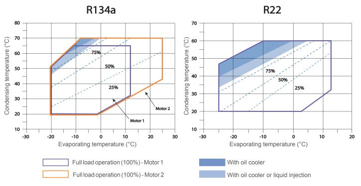
Suction gas superheating 10K - without liquid subcooling.
